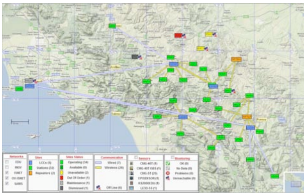
Figure 2. A snapshot from the ISNet Database in which is shown the ISNet topology and communication links.
