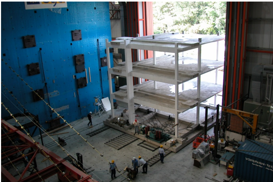
Figure 1. Pre-Normative Test being carried out on an existing RC building for the calibration of Eurocode 8.
