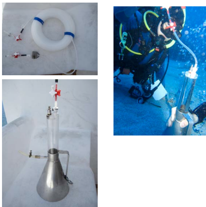
Figure 1. Stainless steel funnel with gas separation chamber, gas hose with 3-way valve, and funnel during sampling.
