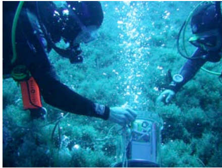
Figure 2. Installation of the CO 2 /H 2 S sensor by divers.
