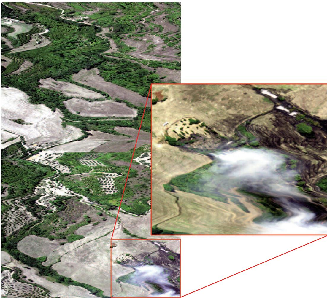
**Figure 2** TVNIR True Colour composition. R=ch.198, 621.15 nm; G=ch.153,569.09 nm; B=ch.92, 499.81 nm plus sub area selected.
