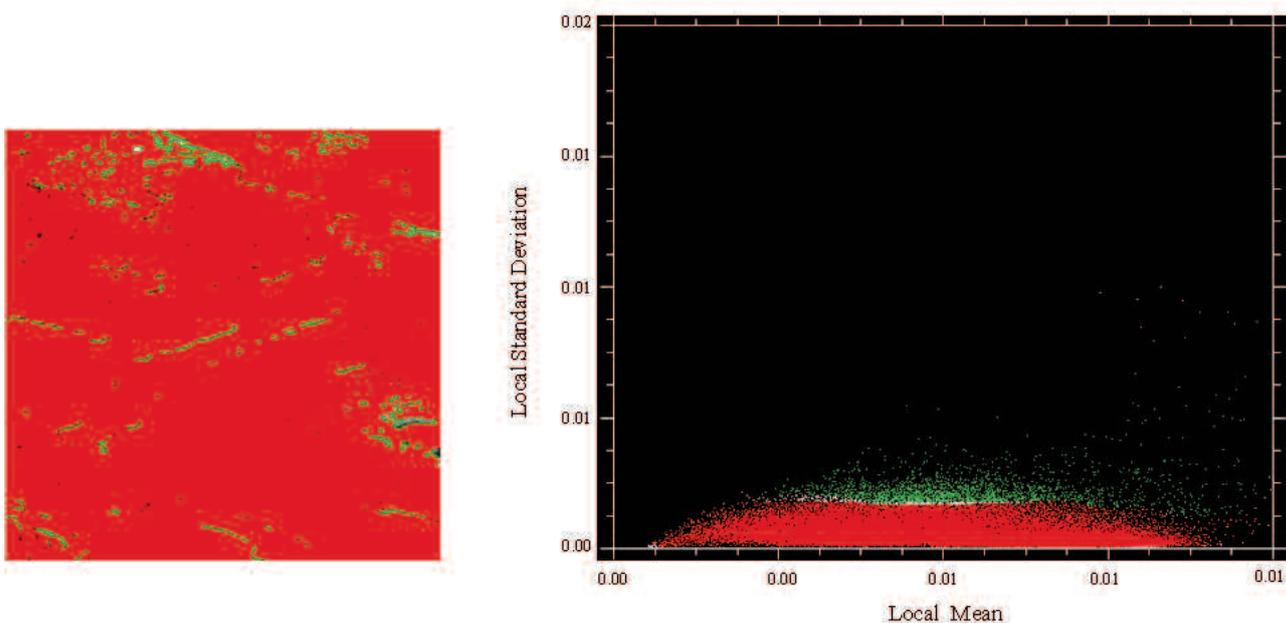
**Figure 6a** SWIR image on left side shows the two clusters: red area corresponds to homogeneous blocks. A scatter plot (on right) of local standard deviations versus local means for a block size 3x3 pixels for the image.
