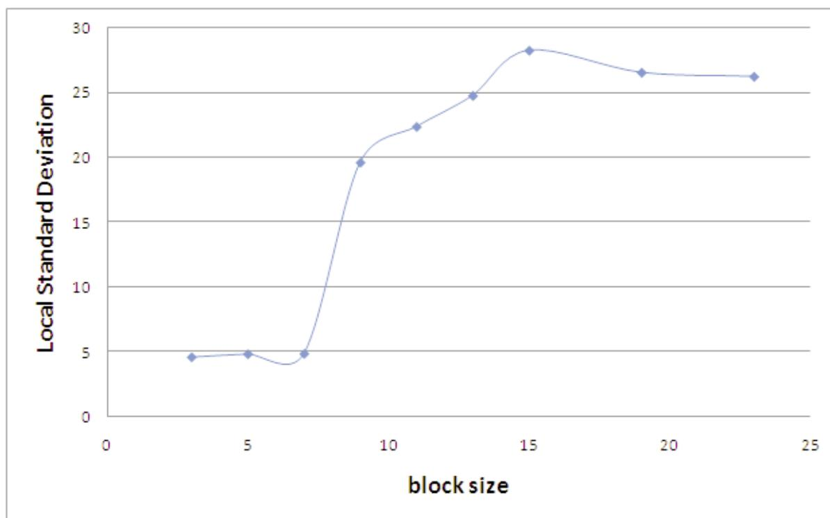
**Figure 3c** LSD estimation varying block dimension.
