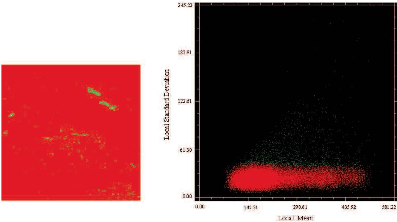
**Figure 5a** The visible image (on the left) shows the two clusters: the red area corresponds to homogeneous blocks, the green area corresponds to inhomogeneous blocks. The scatter plot (on the right) shows the local standard deviations versus local means for a 3x3 pixels block size into the selected image.
