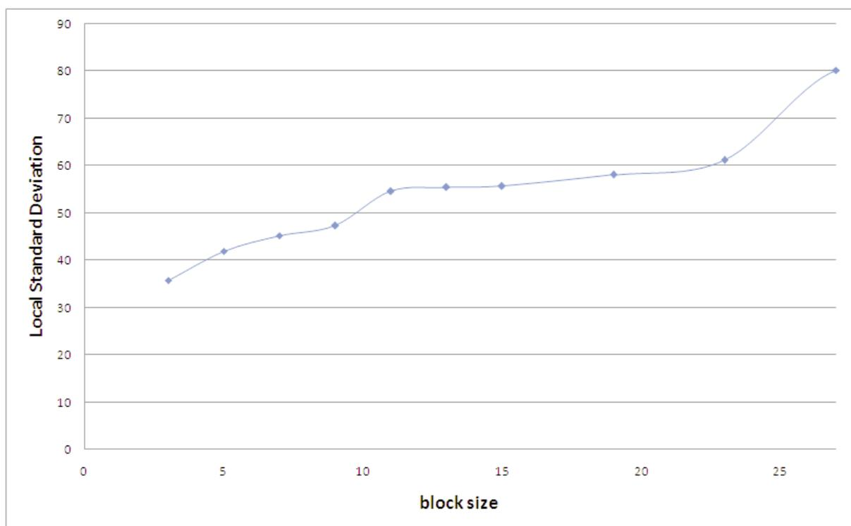
**Figure 4** LSD estimation varying block dimension for test image plus Gaussian noise, band at 569 nm.
