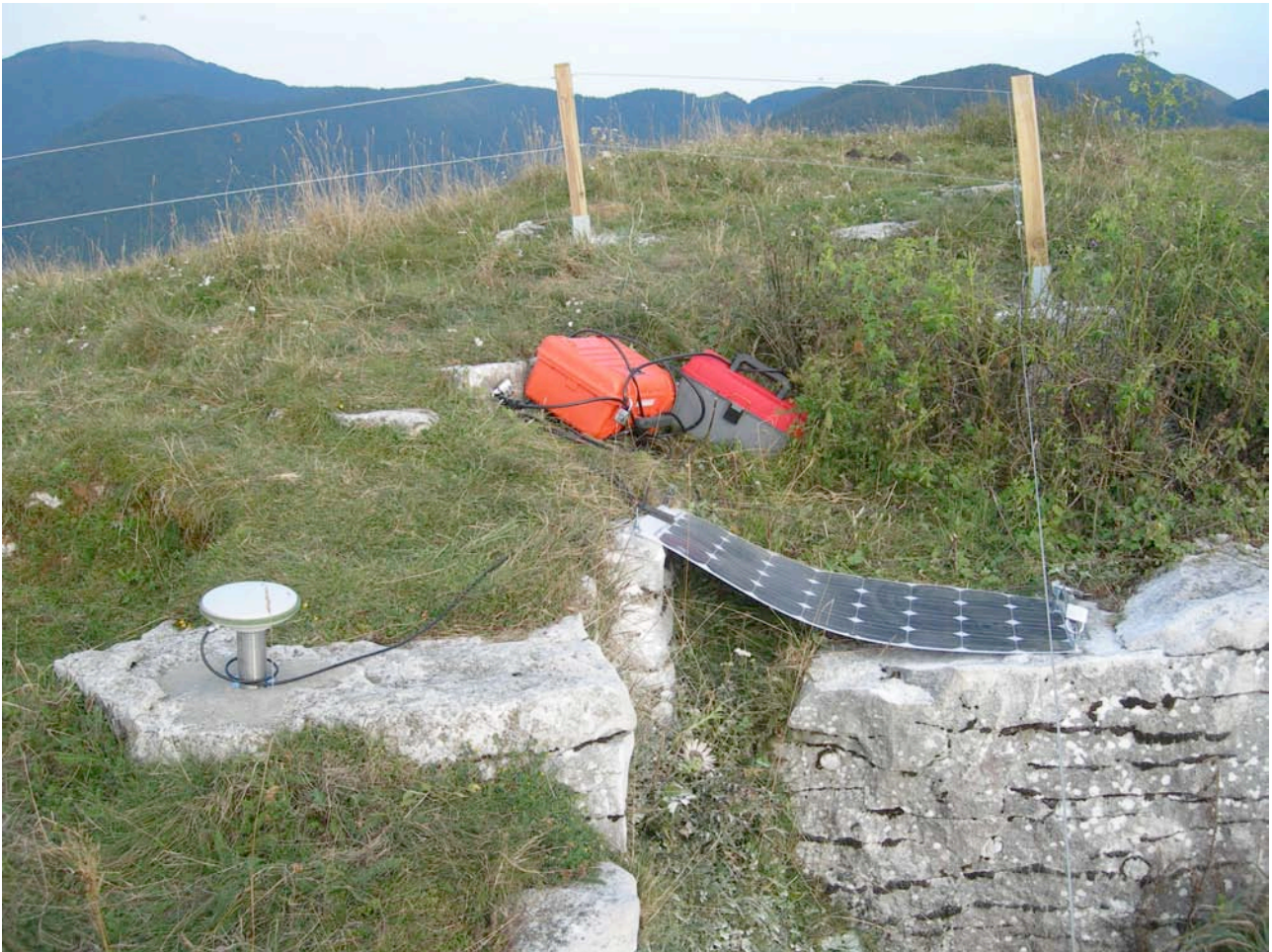
Figure 18. Typical installation and final configuration of a semicontinuous GPS station belonging to our Conegliano-Montello network. The network station book is available in the Appendix A.
