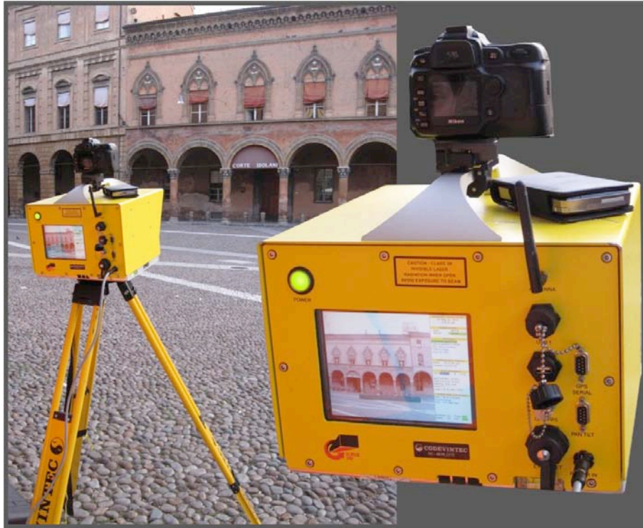
Figure 1. The ILRIS 3D (ER) working in the Santo Stefano square; the external camera (Nikon) is mounted on the scanner handle. The image in the display is the one captured by the internal camera.
