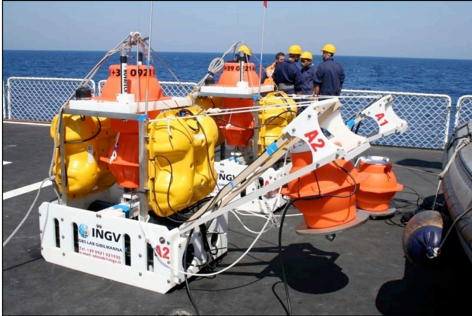
Figure 1 INGV Ocean Bottom Seismometer ready to be deployed in the Ionian sea.
