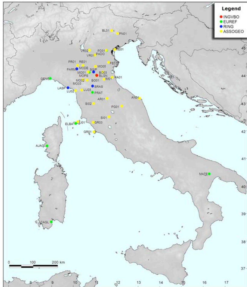
Figure 1 The Italian section of GPS network composed of CGPS belonging to different agencies.
