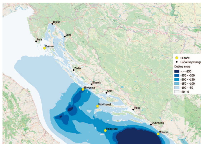
Figure 1 Croatian met-ocean data buoys at East Adriatic; positions and mooring depths.
