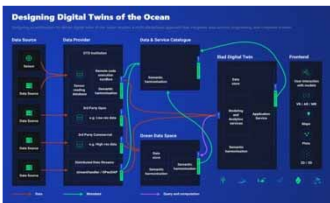
Figure 1 The Iliad logical architecture shows the development pipeline/value chain from data collection on the left to user interface on the right and indicate some of the technologies that are required to build digital twins of the ocean.
