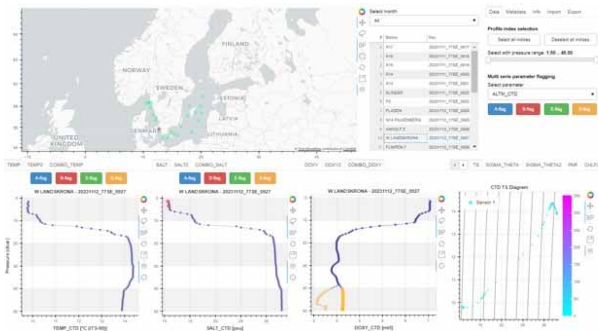
Figure 2 Visualisation of data and automatic quality control results in web browser. Interactive with the possibility to manually flag data.
